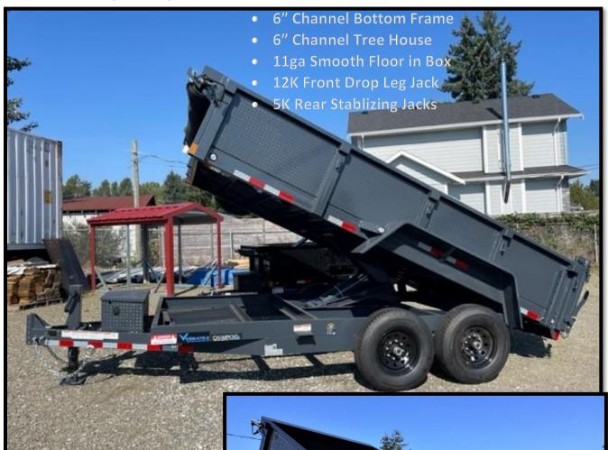
Scissor Lift Hoist -High Lifting Angle Powerful 516 Scissor Lift Hoist
