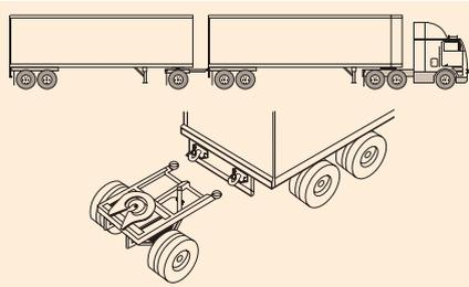
*C train – example of a unit connected by a type C converter dolly.*
