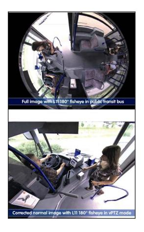
Enlarging or manipulating the image sections within this three-dimensional half sphere gives the impression of a moving camera providing **virtual PTZ** functionality with no moving parts:
