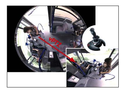
This in-camera hemispheric correction can be applied to multiple image sections. Unlike a mechanical PTZ camera, the Mobotix camera allows multiple areas within a room to be viewed and recorded.
