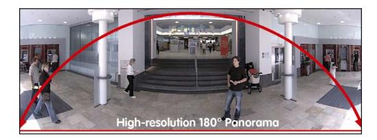
A ceiling mounted hemispheric camera is capable of covering the entire room, generating two  $180^{\circ}$  panoramic views simultaneously:
