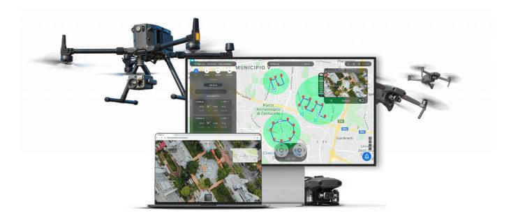
**#5 Add-on Modules:** FlytNow provides add-ons to make a drone intelligent; this includes precision landing over a computer-generated tag, obstacle detection, and object identification. These add-ons enable a drone to autonomously fly to a location, identify a threat, and return to the DiaB hardware.
