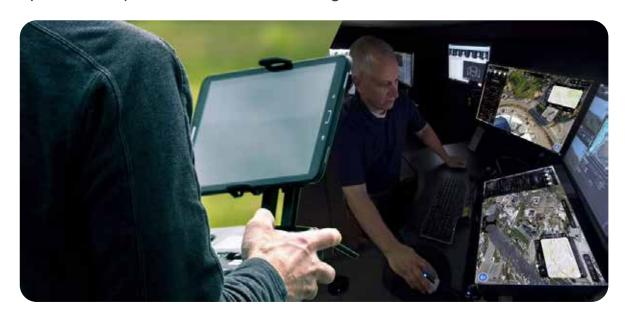
**#3 Live Data Sharing**: An operator can share the live video feed from a drone directly from the dashboard. The feature can be used to share video with the police or other remote stakeholders.
