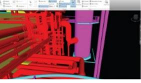
☐ Inspection/Reverse Engineering: Extract measurements and create 3D models when there is no existing CAD data available. Perform detailed inspections and comparisons to existing models, surfaces and point clouds.
