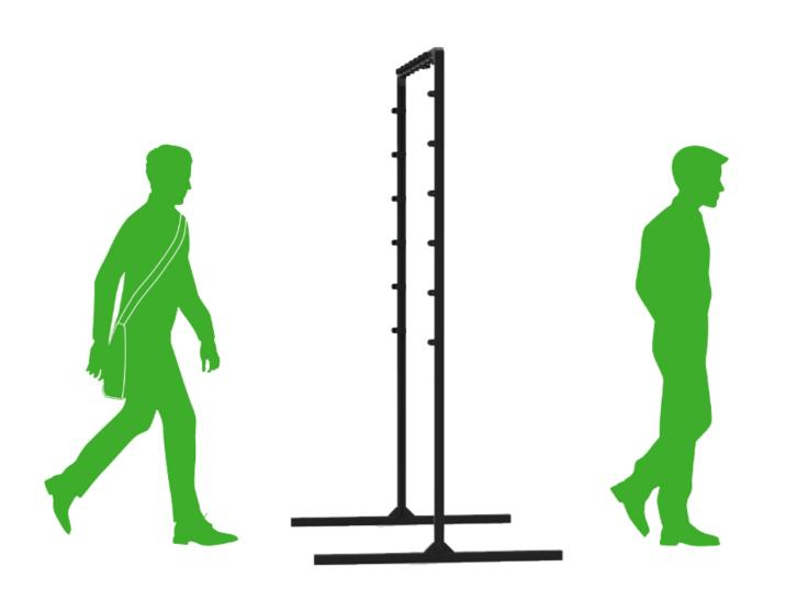
The ThermalPass system detects body temperature using touchless, infrared, thermal medical grade sensors, while identifying potential at-risk carriers.
