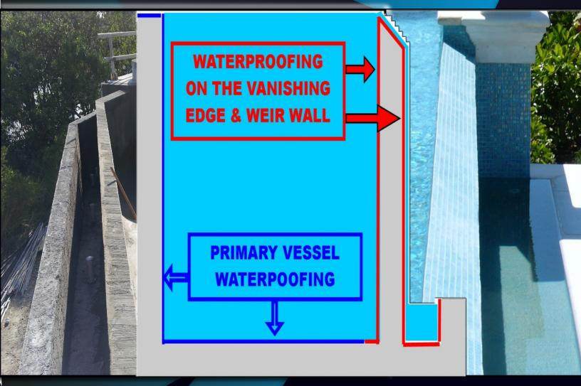
Vanishing edge pools have become an important water feature in both commercial and residential applications. Flexcrete cement based waterproofing membrane enhances and preserves the look by eliminating the possibility of unsightly efflorescence on tile grout lines while waterproofing the entire structure with integrity and permanence.
