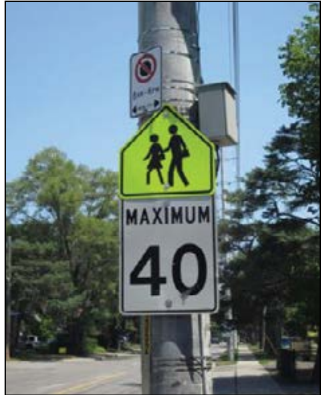
Figure 79 – Example of Municipal Sign Grouping (two regulatory signs and a warning sign)
