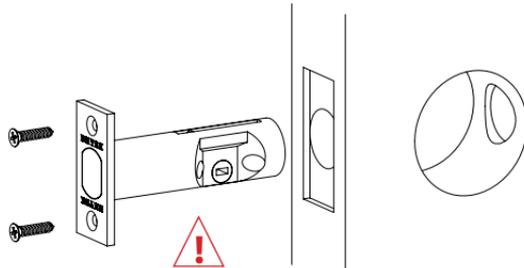
Note: Use only the supplied latch for proper functionality.
