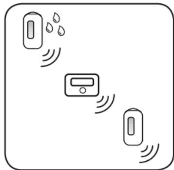
Each sensor will also act as a repeating station during alarm conditions, so any signal received by a device will be rebroadcast.
