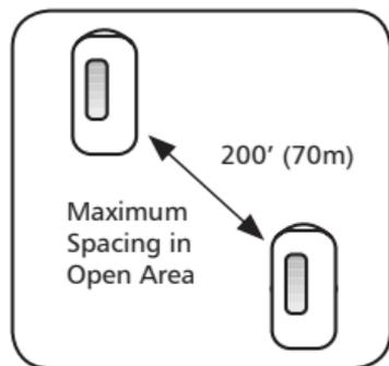
The sensor-to-sensor radio communicates using radio frequencies between 905.2MHz and 913.2MHz. The range of this radio has been tested to 200 ft (70m) in open area distance testing. The Comm Link's WiFi communicates at 2.4GHz, which produces a shorter indoor range.
