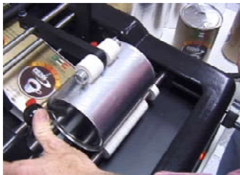
Insert container and tap lever to apply label.
