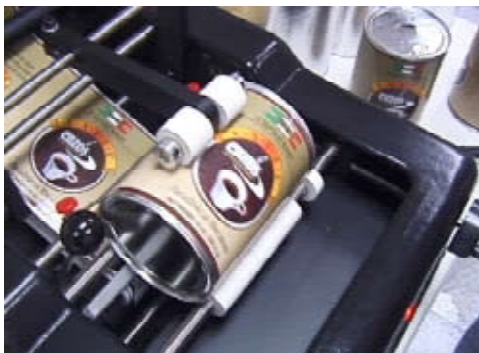
Label is applied within seconds, up to 25 cps.
