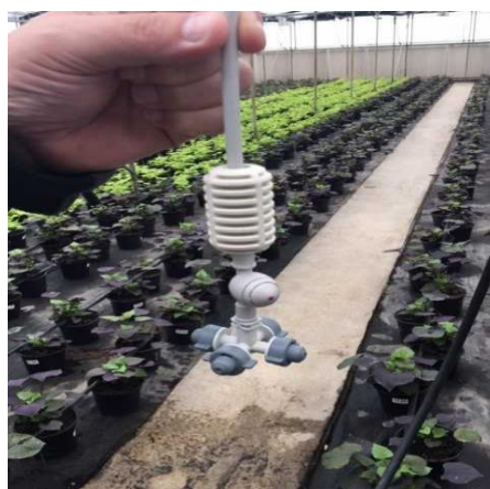
Foliar Spray Nozzle equipped with CO2 diffusion
