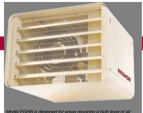
Model EGHB is designed for areas requiring a high level of air flow. This unit heater may be mounted horizontally (wall or ceiling) using supplied brackets or vertically using 4 threaded rods.
